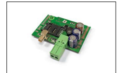
Modem GSM e internet GPRS (COMAP) GSM modem and internet GPRS (COMAP) Modem GSM et internet GPRS (COMAP) Modem GSM e internet GPRS (COMAP)
